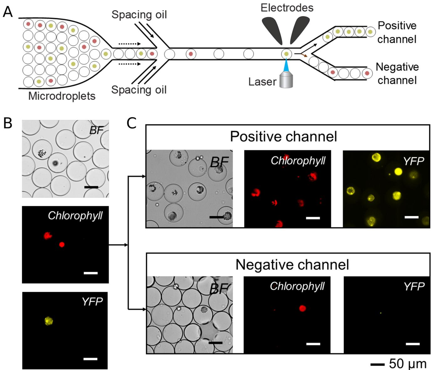
**Fig 6. Sorting of *M. polymorpha* protoplasts.** (A) Schematic representation of a platform for microfluidic sorting of encapsulated protoplasts. (B) Bright field and fluorescence micrographs of adjacent microdroplets containing protoplasts derived from wild-type and transgenic *mpt0 M. polymorpha*, respectively. (C) Bright field and fluorescence micrographs of microdroplets sorted into positive and negative channels based on their mVenus fluorescence intensity.
