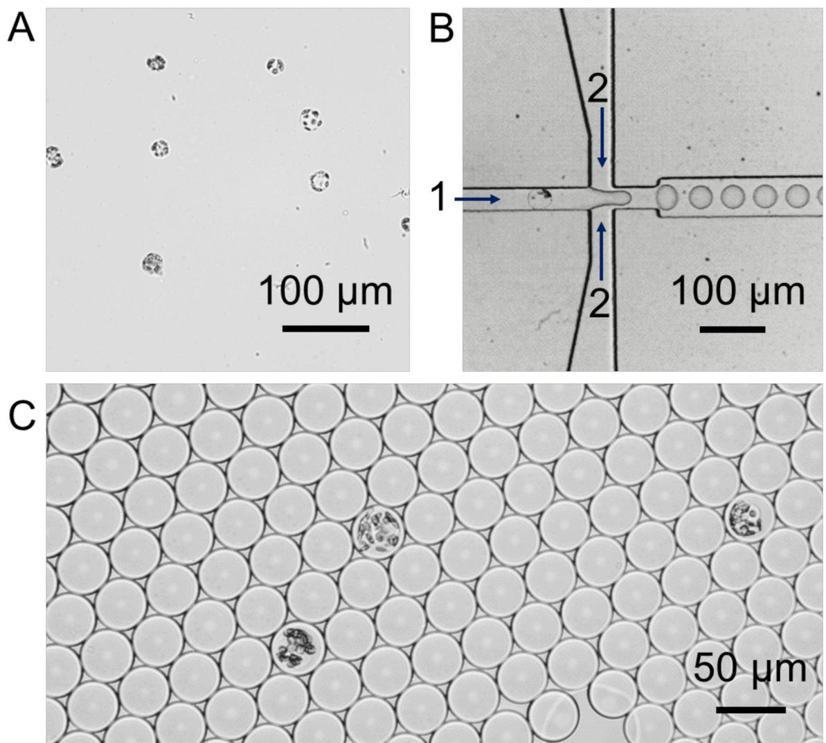
**Fig 1. Encapsulation of *M. polymorpha* protoplasts.** (A) Bright field micrograph of *M. polymorpha* protoplasts isolated from mature thalli. (B) Bright field micrograph of a flow-focusing microfluidic device for encapsulation of *M. polymorpha* protoplasts in water-in-oil microdroplets. (C) Bright field micrograph of individual *M. polymorpha* protoplast encapsulated in microdroplets.
