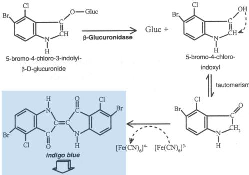
Fig. 1. Chemistry of X-Gluc reaction. Hydrolyzation of X-Gluc by the  $\beta$ -glucuronidase enzyme results in a reactive indoxyl molecule. Two indoxyl molecules are oxidized to indigo blue; ferri(III)cyanide enhances the dimerization.
